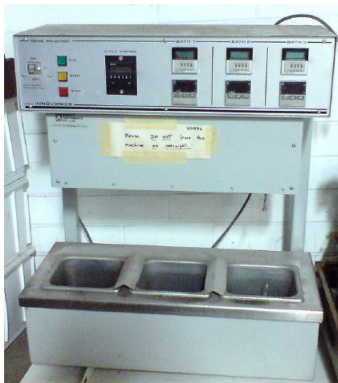
Fig. 7.1 An older, three-temperature thermal cycler for PCR
