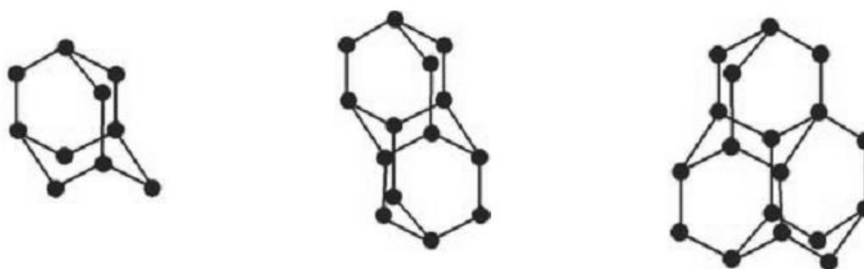
Figure: Molecular structures of adamantane, diamantane and triamantane, the smaller diamondoids, with chemical formulas \text{C}_{10}\text{H}_{16} , \text{C}_{14}\text{H}_{20} and \text{C}_{18}\text{H}_{24} , respectively.
