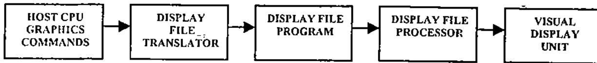
Figure 10: Block Diagram of Line Drawing Display
